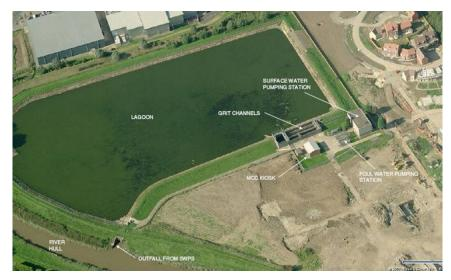
7.1.3 In contrast to the rest of Hull, Bransholme has separate systems to deal with surface water and sewage.
