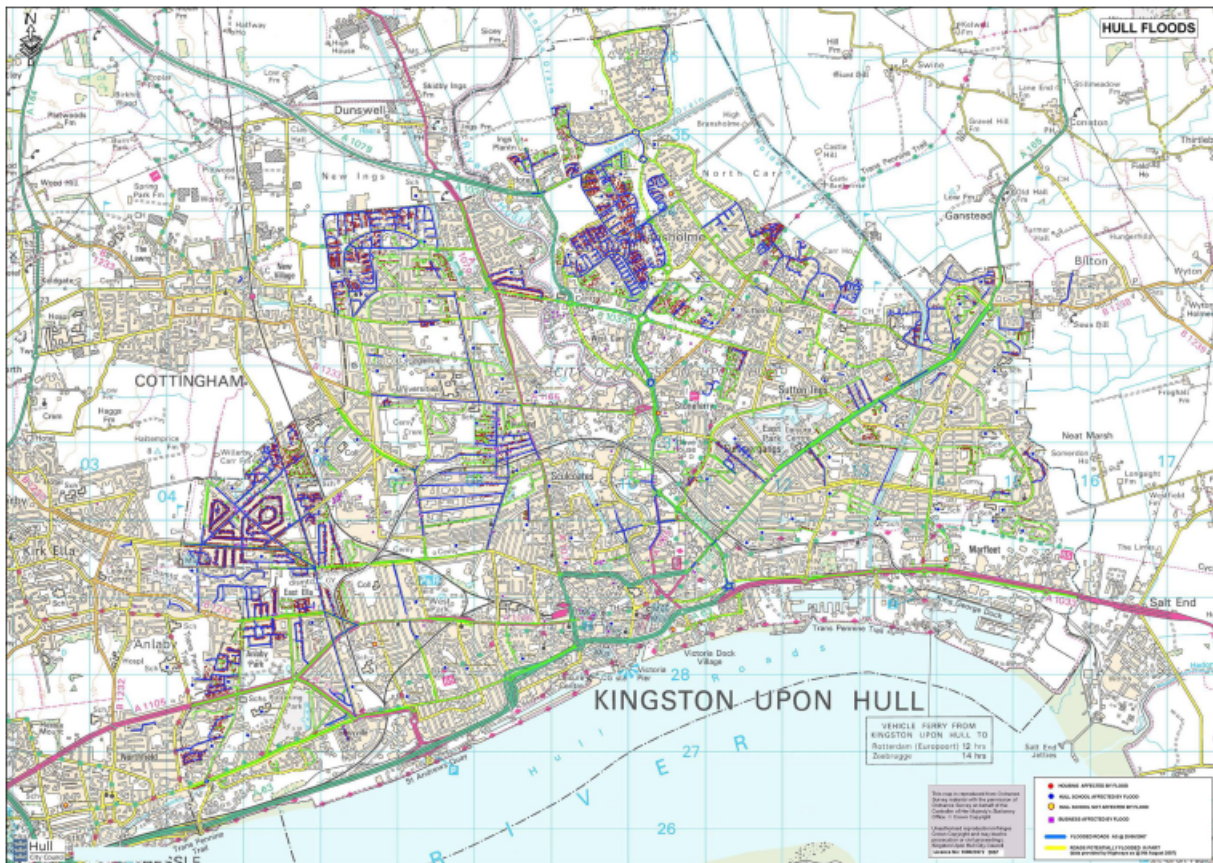
Figure 5 Areas in Hull flooded. Lines correspond to flooded roads and dots show flooded properties.
