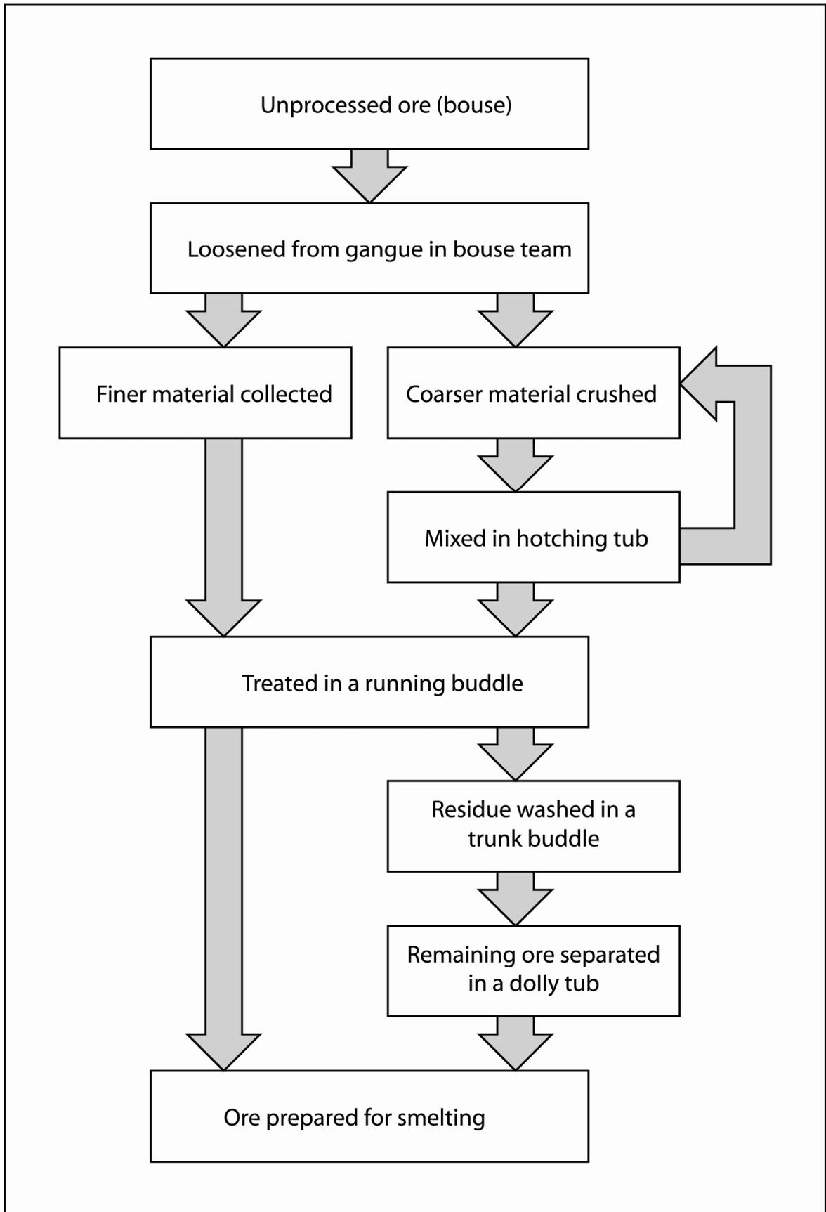
Figure 2.6: The ore dressing process employed in Swaledale lead mines
